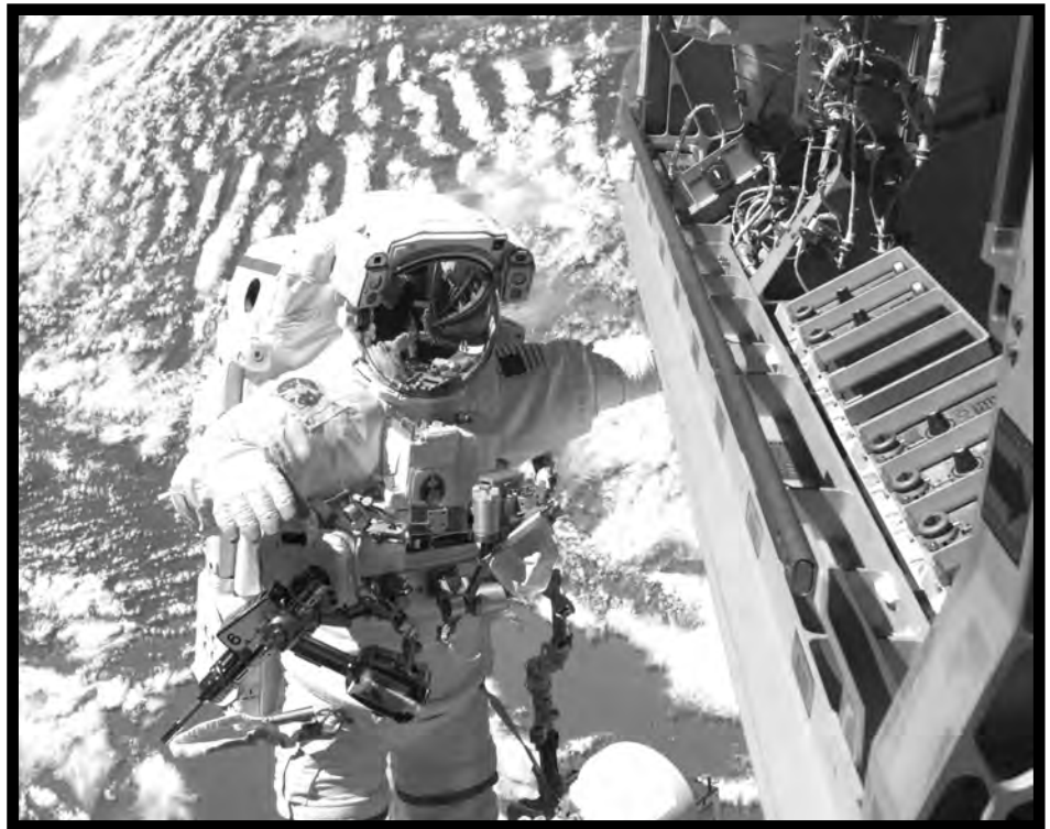
No sweat—you could ride there and back. Astronaut Robert L. Curbeam Jr. prepares to replace a faulty TV camera on the exterior of the International Space Station during a December 2006 mission. Photo courtesy of NASA.
